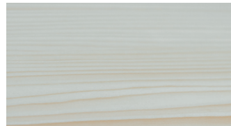
LEACHED AND SOAPED SPRUCE
