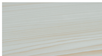
LEACHED AND SOAPED SPRUCE
